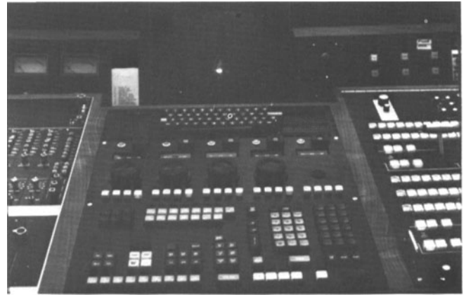
Fig. 2. Three-part control panel. (Top) alphanumeric keyboard; (Middle) joystick control knobs; (Bottom) main control panel.
