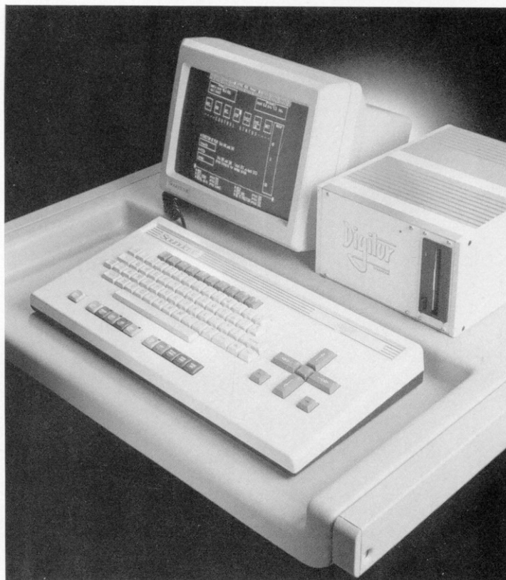
Fig. 11 Soundcraft Digitor is a solid-state recorder-editor using large RAM. RAM capacity limits recording time, but access to any part of recording is immediate, speeding editing process. RAM is volatile; work must be dumped to storage medium afterward.
