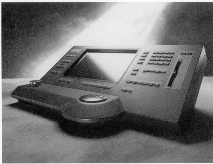
Fig. 9. Digital Audio Research offers the Soundstation II hard-disk-based editor. It uses touch screen controls to enhance rapid access of disk drives.
