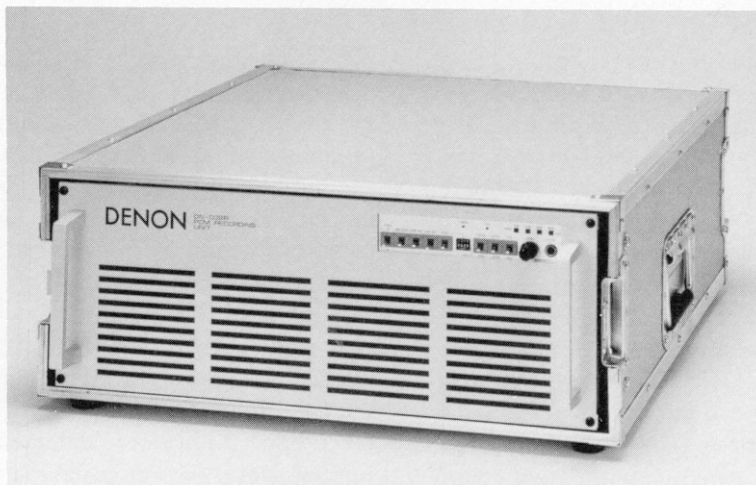
Fig. 4. The Denon DN-039R PCM adapter allows simultaneous recording of four digital audio channels on a video cassette recorder.
