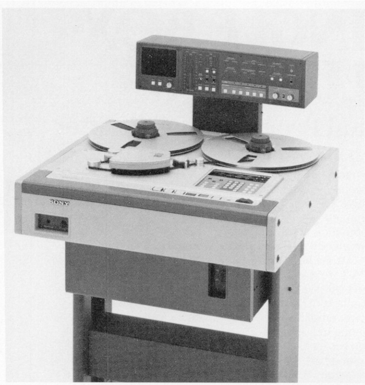
Fig. 8. Sony PCM-3402 is a two-speed DASH machine. At 7.5 in/s it records two channels in normal DASH for tape economy and long play time. At 15 in/s it records two-channel TWIN DASH, which has better performance for tape-cut splicing.
